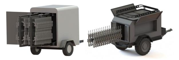
Trailes are sized and built to meet customer's requirments, including armorers workbench, lighting, 120v/12v power, cleaning station, support gear storage, desrecte exterior apearacne or customized exterior graphics.
